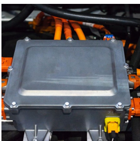
Battery Management Systems
