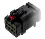
terminal strength, 13A current rating, lanceless design and a wide wire range of 20-14 AWG. The TE Connectivity AMPSEAL 16 connector system is available in 2-12 positions and features keying/polarization to prevent mismating. The system also includes integral CPA and TPA mechanisms to ensure connector and terminal positioning for secure mating.
