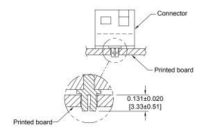
MATERIAL: Spring tempered copper alloy, tin plated.
