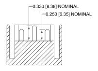
MC610NS and MC612N crimp contacts and MC610NS and MC612N solder cup contacts to be used for 0.330 [8.38] nominal mating length. MC610NS-228.2 and MC612N-228.2 crimp contacts and MS610NS-228.2 and MS612N-228.2 solder cup contacts to be used for 0.250 [6.35] nominal mating length.
