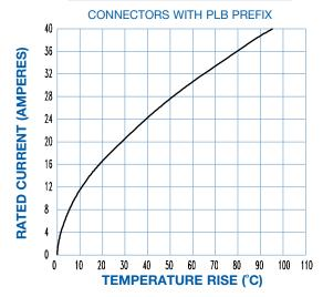
Test conducted per IEC Publication 60512-3, Test 5a.
