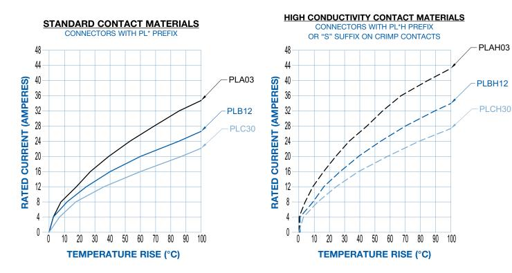
**TEST DETAIL:** Each curve was developed using individual connector bodies fully loaded with contacts. All power contacts energized through 12 awg wire. Temperature rise was measured in the contact mating area. Test was conducted with connectors in static air. Terminations of test connectors were straight compliant press-in to right angle (90°) solder. See page 4 for more information.
