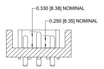
Modification number -338.0 (see step 8 of the ordering information) allows for board mount connector to have position 3 loaded with a 0.330 [8.38] nominal mating length contact and positions 1 and 2 loaded with 0.250 [6.35] nominal mating length contacts. Contact technical sales for additional sequencing options.
