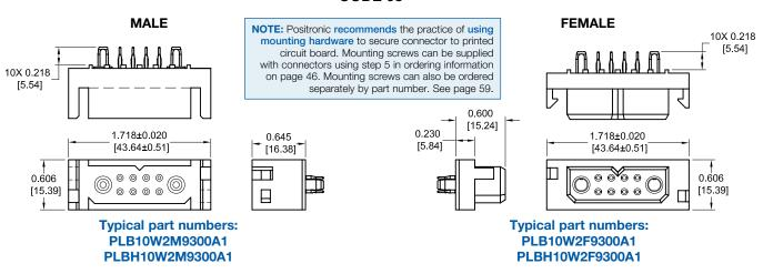
NOTE: Connectors are designed to be mounted to the printed circuit board with screws, see page 59 for mounting screw information. See page 43 for contact hole pattern.
