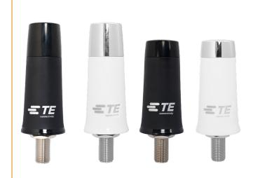
The 5G Phantom NGP antenna series cover either 617-7125 or 698-7125 MHz in a ground plane independent format. Offering global cellular coverage, without the need for a fixed ground plane, even for regions where the lower 600 MHz band is required. They deliver high levels of average efficiency, over 95% up to 4200 MHz, and gain up to 8.0 dBi in an IP67-rated, compact form factor.
