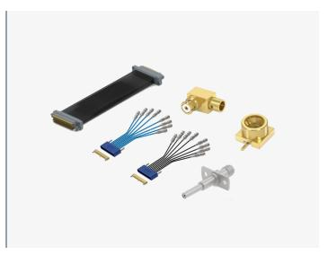
TE Connectivity's Blind-Mate Coaxial Products consist of a portfolio of solutions including SMP/SMPM, Test Probes, Multi-Port and Massive Coaxial, allowing for a wide range of applications. With frequencies ranging from 1.60GHz to 67GHz and reliability testing up to 10,000 cycles, Blind-Mate products provide RF testing and signal sampling where space and visibility are minimal.
