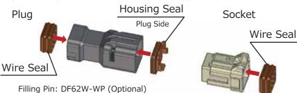
Insert the filling pin into the contact cavity.
